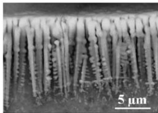
Fig. 2 Formation of dendrites of  $\delta$ -TiN<sub>x</sub> after bursts of FEL irradiation at 3.15 microns. From Ref 19
