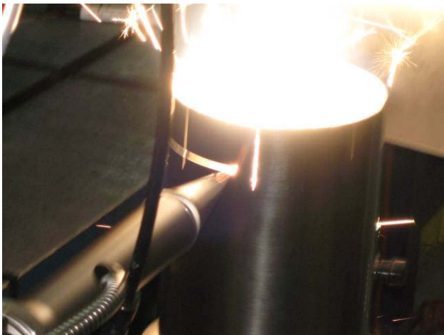
Figure 3a: A Fugen Zirconium alloy pressurized tube of about 4.3mm thick and 117.8mm inner diameter was successfully and quickly cut with 6m per a minute using 20 bar compressed and focused N 2 gas flow and IPG 5kW fiber laser.
