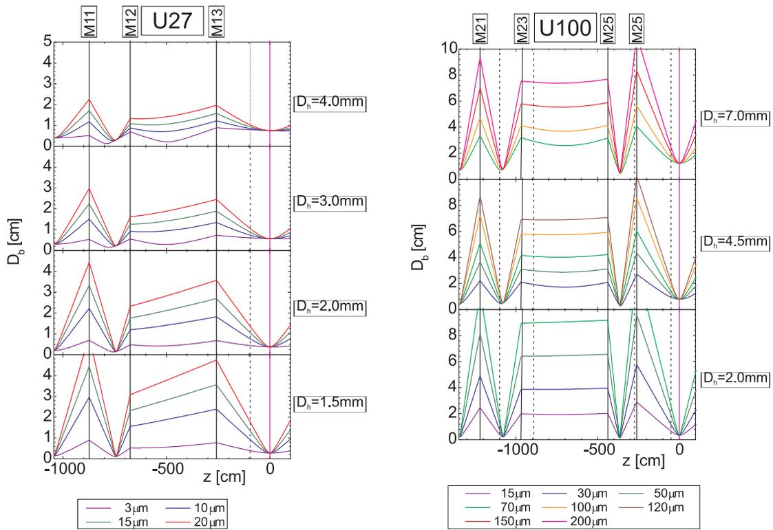
Figure 3: Diameter  $D_b$  of the IR beam calculated along the beam line from the outcoupling hole to the waist on the diagnostic table ( $z=0$ ) for various wavelengths and outcoupling holes with diameter  $D_h$ . Focusing (Mik) and flat mirrors are indicated by vertical solid and broken lines, respectively. The position of the diagnostic waist is indicated by the magenta line. Left panel: U27-FEL, right panel: U100-FEL.
