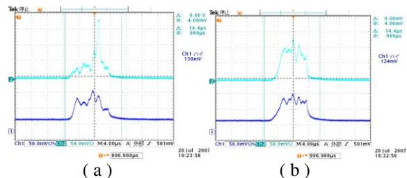
Figure 6: Macropulse waveforms of fundamental and second harmonic: (a) fundamental (lower trace) and nonlinear harmonic (upper trace), (b) fundamental and SHG.
