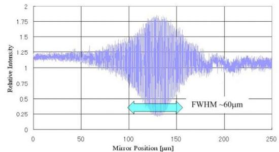
Figure 3: Autocorrelation trace at the wavelength of 1500nm.
