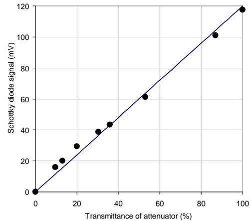
Figure 3: Signal of the Schottky diode detector versus transmission of the attenuator for working conditions of the detector.
