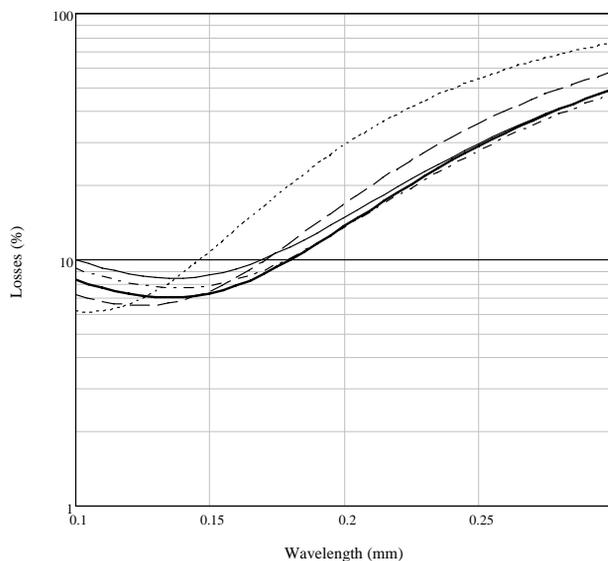
Figure 2: Total losses per round trip of NovoFEL versus wavelength for different Rayleigh lengths:  $L_f = 3$  m (dotted line),  $L_f = 4$  m (dashed line),  $L_f = 5$  m (thick solid line),  $L_f = 6$  m (dash-dotted line),  $L_f = 7$  m (thin solid line).
