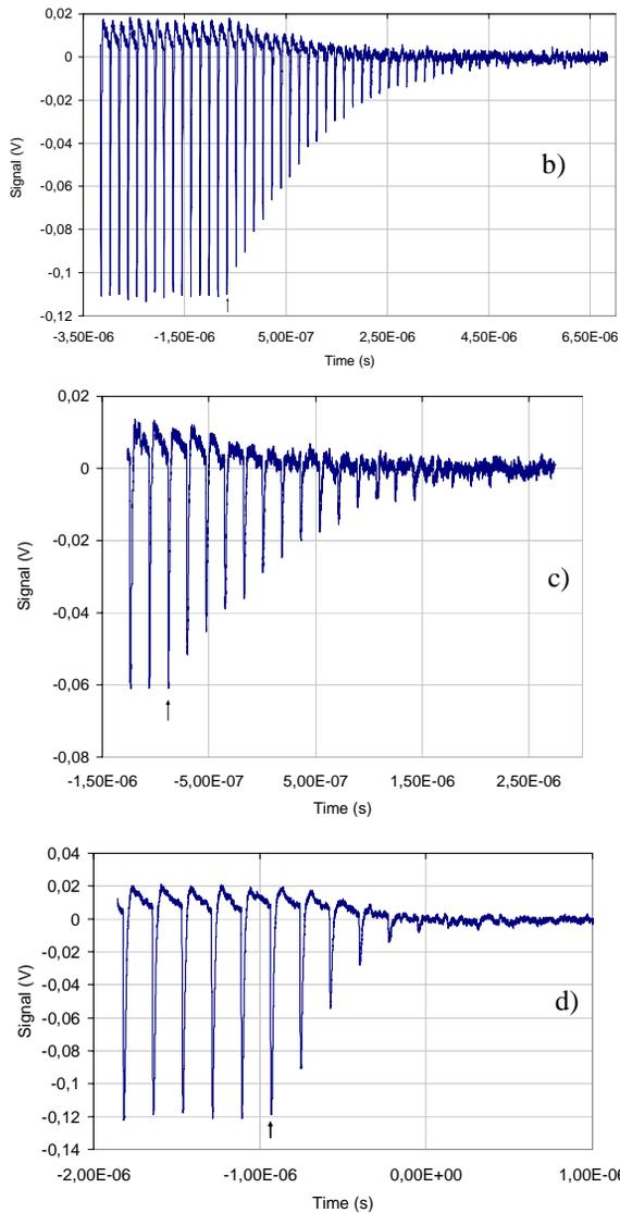
Figure 4: Time evolution of NovoFEL light pulses after switch-off of electron pulses for radiation with different wavelengths: 152.5  $\mu\text{m}$  (b), 197.3  $\mu\text{m}$  (c), and 229.4  $\mu\text{m}$  (d). Switch-off time is shown by arrows.
