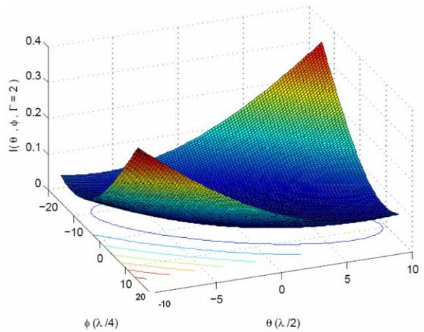
Fig. 3. The intensity with ‘crossed polarizer scheme’ when  $\Gamma$  is 2 degree.  $\theta$  is the angle of half wave plate for compensation and  $\varphi$  is the angle of quarter wave plate. Note that y axis is normalized by the initial laser intensity.
