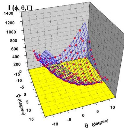
Fig. 4. The intensity with ‘crossed polarizer scheme’ measured in FLASH.  $\theta$  is the angle of half wave plate for compensation and  $\varphi$  is the angle of quarter wave plate. Note that y axis is not normalized by the initial laser intensity. The unit is same with the Fig. 2 i.e. the ICCD unit.
