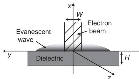
Figure 1: Geometry used for the three-dimensional model. The electron beam has a width  $W$  and is allowed to extend to infinity in  $\hat{x}$ . The dielectric had a depth  $H$  and is wide compared to both the evanescent scale height and mode width.
