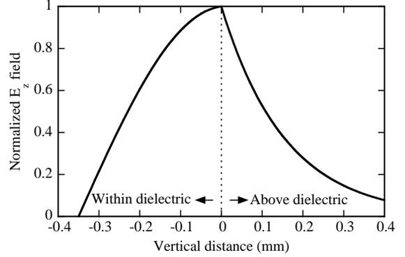
Figure 5: Vertical profile of the electric field. The field height is much smaller than the field width shown in Figure 6.
