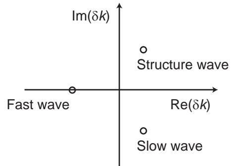
Figure 3: Roots of the dispersion relation for a wide electron beam. These are the same as for the two-dimensional result.
