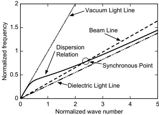
Figure 2: The two-dimensional dispersion curve for the parameters used in experiments at Dartmouth (see Table 1). Only the first order branch is shown.
