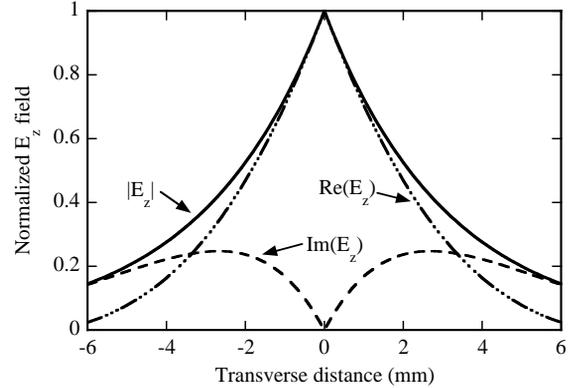
Figure 6: Transverse profile of the electric field. The field is much wider than the electron beam used in experiments. It is also wide compared with the evanescent scale height.
