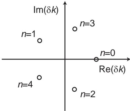
Figure 4: Roots of the dispersion relation for a narrow electron beam. Because of physical constraints, only  $n = 2$  and  $n = 3$  roots are true solutions. The  $n = 2$  root has positive gain, while  $n = 3$  has negative gain. Both modes have the same width and are slow waves ( $\text{Re}(\delta k) > 0$ ).
