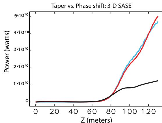
Figure 6: Power for normal (black), tapered (red) and phase-shifted (blue) LCLS-like SASE FEL, 3-D simulation. 12 Phase shifts between undulator sections (3.8 m).
