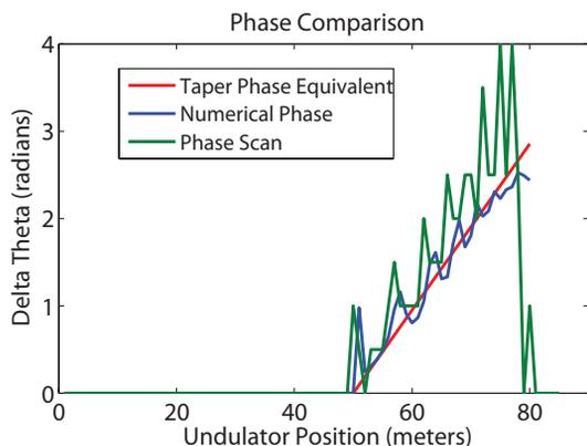
Figure 4: Phases determined by phase scan, numerical optimization and taper equivalent (Seeded case).
