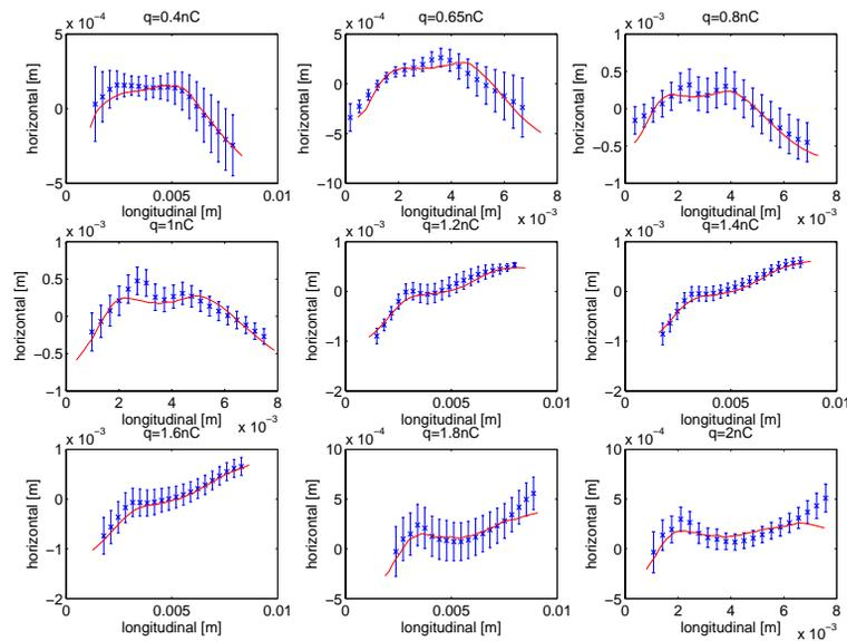
Figure 5: Comparison of centroid curves obtained from measurements (blue) and simulations (red). ACC1 phase offset is  $\varphi = 24.9^\circ$ . The centroid curves obtained by the image analysis of measured profiles are shown. Bunch heads are to the left.
