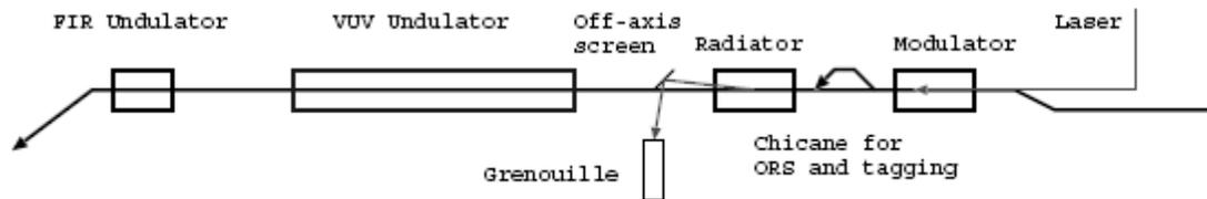
Figure 1: Schematic view of the Optical Replica Synthesiser.
