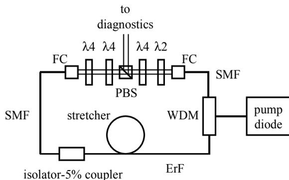
Figure 2: Schematic view of the Erbium fiber oscillator. FC: fiber coupler; SMF: single mode fiber; ErF: Erbium doped fiber, PBS: polarising beam splitter, WDM: wavelength division multiplexer,  $\lambda/4$ : quarter lambda plate,  $\lambda/2$ : half lambda plate.
