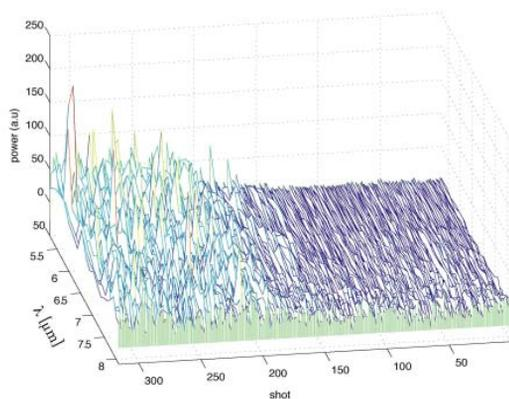
Figure 12: A set of successively recorded single shot spectra in the wavelength range 5-8  $\mu\text{m}$  from coherent transition radiation at FLASH. While recording from right to left, the off-crest phase of the first accelerating module was scanned from zero to about -8 degrees.
