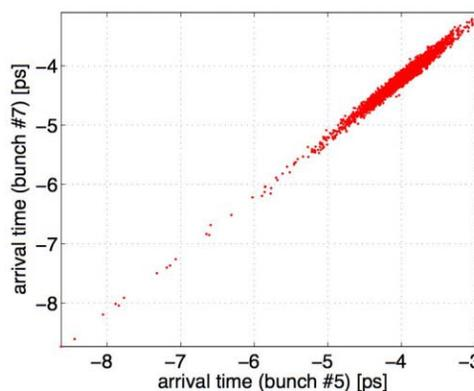
Figure 2: Time difference between two bunches of the same bunch train at FLASH, measured with a phase monitor using electro-optic detection of the zero crossing of a pick-up signal. The combined time jitter and monitor resolution is of the order 50 fs[12].
