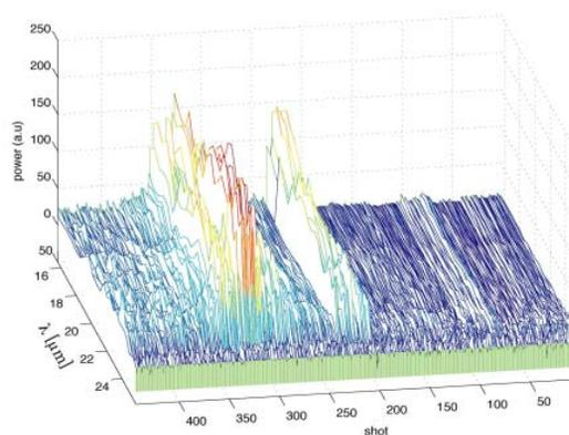
Figure 11: A set of successively recorded single shot spectra in the wavelength range 16-26  $\mu\text{m}$  from coherent transition radiation at FLASH. While recording from right to left, the off-crest phase of the first accelerating module was scanned from zero to about -8 degrees.
