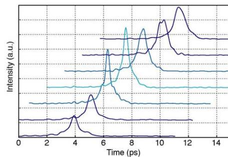
Figure 7: Single shot bunch profiles measured with electro-optic spatial decoding at the SLAC-FFTB using a ZnTe crystal [22].
