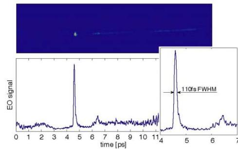
Figure 9: Longitudinal bunch profile measured at FLASH with the electro-optic temporal decoding technique using a  $100\mu\text{m}$  thick GaP crystal [24].
