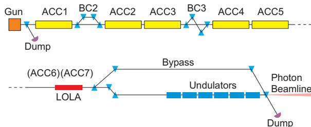
Figure 1: Sketch of FLASH. The blue triangles indicate dipole magnets, the yellow boxes TESLA acceleration modules.
