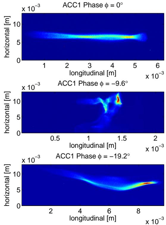
Figure 4: Measured top view for different ACC1 phase off-sets. Top: no compression. Middle: near full compression. Bottom: over-compression.
