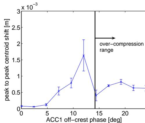
Figure 5: The peak to peak centroid shift along the bunch is plotted vs. the phase offset in ACC1. Phase range used for the experiment: 14 to 24 degrees.
