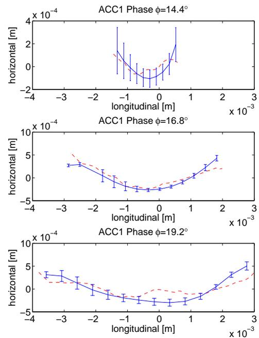
Figure 7: Experimental centroid curves are compared with simulated data. The blue lines represent the data taken with LOLA and the dashed red curves represent the results of simulations. Linear correlations are subtracted.
