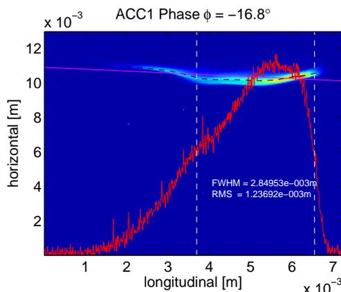
Figure 2: An example of a LOLA measurement. Longitudinal charge profile (red line), fwhm and rms bunch length are shown.
