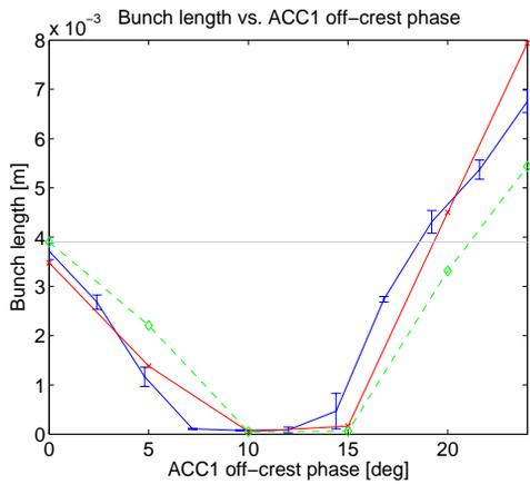
Figure 3: Measured fwhm bunch length at LOLA (blue line) are compared with simulations. Red line: calculated bunch length at LOLA. Green line: calculated bunch length after BC2.
