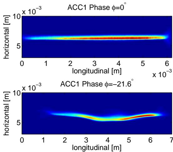
Figure 6: Simulated top view after BC2 for different ACC1 phase offsets. Top: no compression. Bottom: over-compression.
