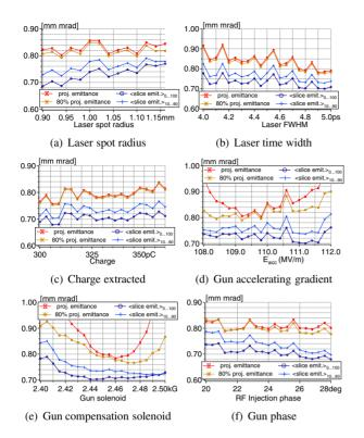
Figure 5: Sensitivity studies: emittance behavior vs. laser and gun parameters.
