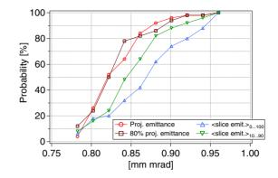
Figure 6: Each point refers to the probability to have a projected emittance less than the value on the x-axis.
