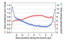
Figure 4: Slice emittance and slice energy spread along the bunch at the exit of SOB.
