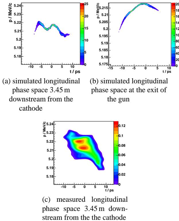
Figure 7: Simulated longitudinal phase space for optimum launch phase, flat-top laser distribution and about 40 pC bunch charge at dipole position (a) and at the exit of the gun (b). In (c) the measurement result is displayed.
