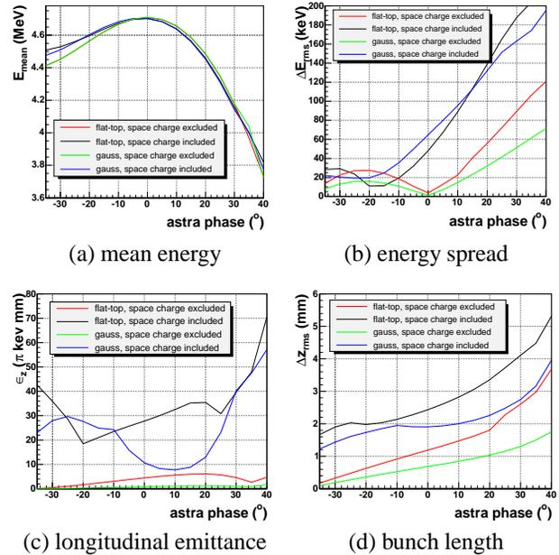
Figure 6: Simulated mean energy (a), energy spread (b), longitudinal emittance (c) and bunch length (d) as a function of the launch phase.
