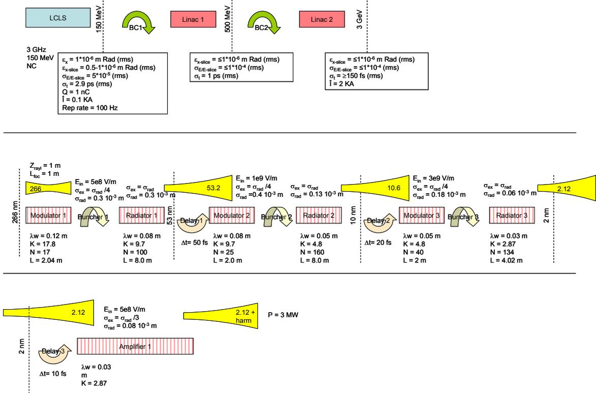
Figure 1. Schematics of the linacs and optical klystrons
