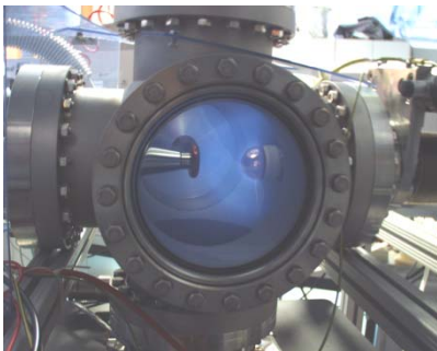
Figure 4: Picture of the high gradient test stand during helium glow discharge treatment used for cleaning / polishing the electrodes.
