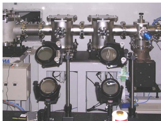
Fig. 4. The picture of the FEL monitor chambers and associated optics on the optical base. Each chamber contains a \text{CaF}_2 beam sampler and a total reflection mirror for an alternative use.
