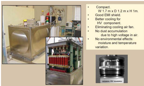
Fig. 2. Klystron pulse modulator for SCSS project. All HV components are installed in metallic shield tank, and filled with oil.
