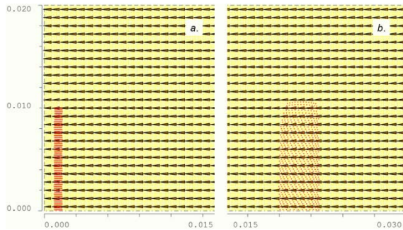
Figure 4: Electron bunch near the photocathode ( a. t=0.08 ns, E_{\max}=5.3 MV/m; b. t=0.24 ns, E_{\max}=9.4 MV/m).
