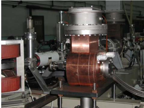
Figure 9: Picture of the new RF-gun.
