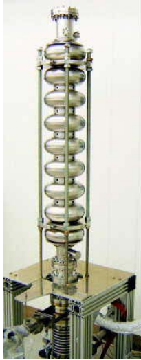
Figure 2: High pressure rinsing of a nine cell 1300 MHz TESLA cavity at ACCEL.
