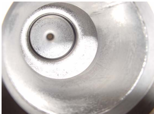
Figure 3: 1+1/2-cell cavity after DC sputtering.
