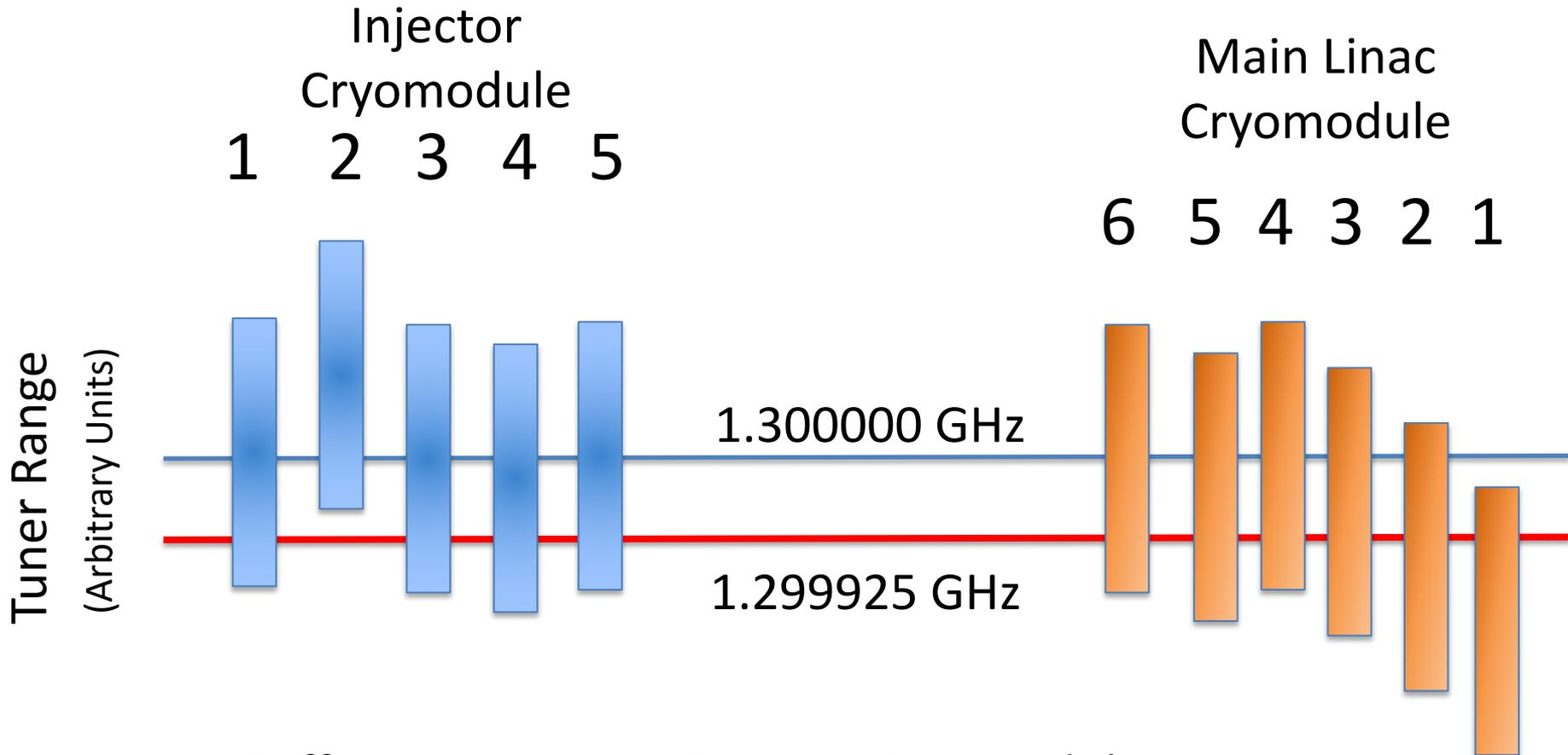
Sufficient margin in Injector Cryomodule to run
