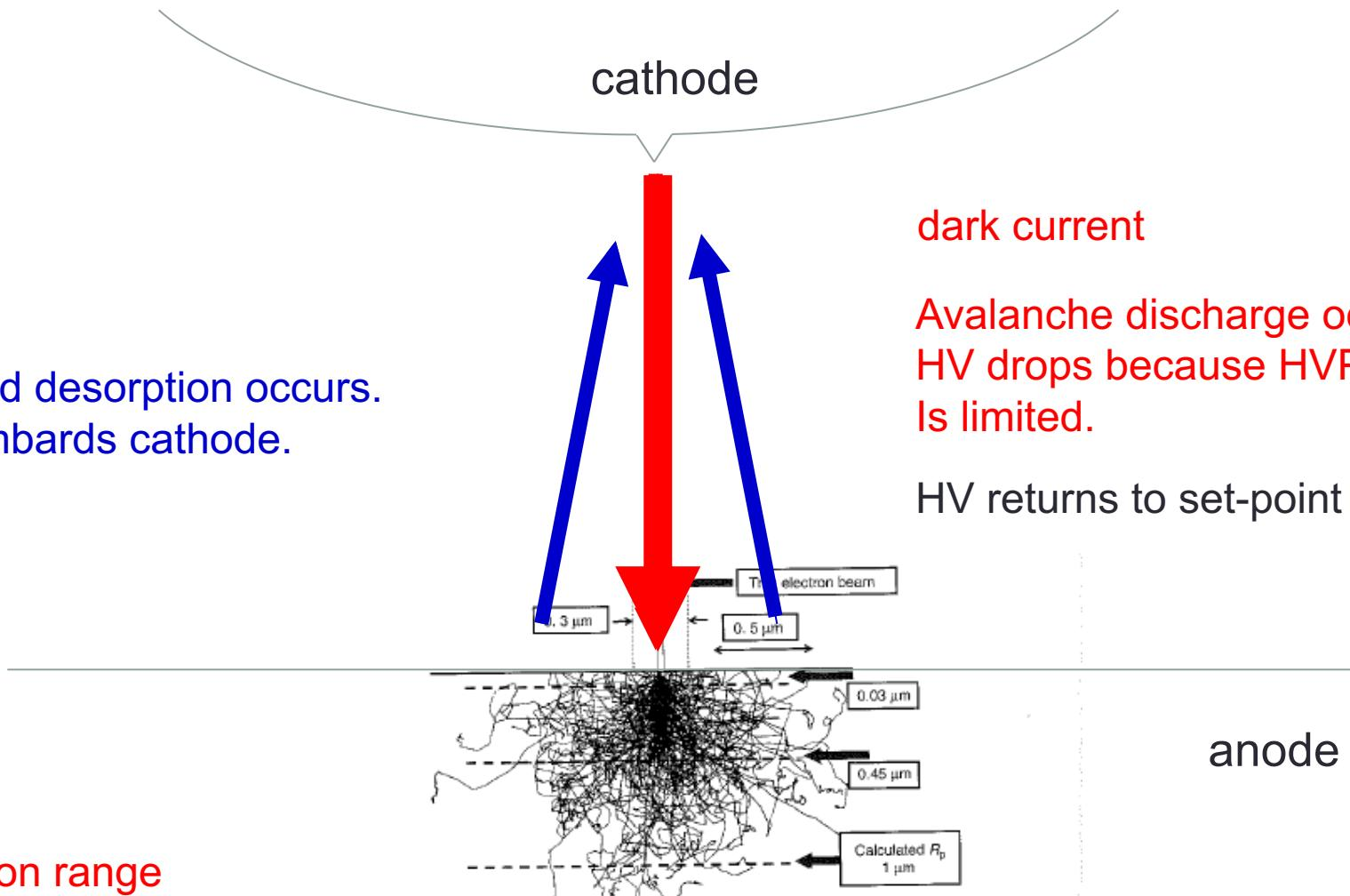
FIGURE 1.49 Monte-Carlo simulation of a thin, 20 keV electron beam at normal incidence on to an Fe anode [84].
