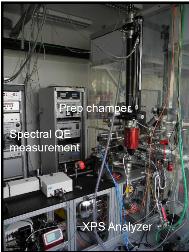
Preparation & Analysis System (PAS) w/ spectral response setup
