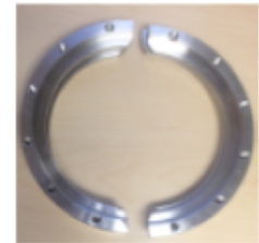
NbTi flanges (completed)
