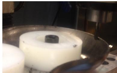
Endgroup equators machined at interior to achieve nearly uniform thickness
