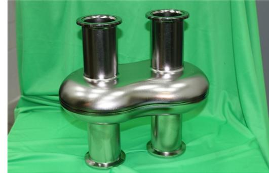
1<sup>st</sup> prototype twin-axis cavity made from high RRR Nb (cavity #1)
