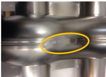
2<sup>nd</sup> prototype cavity after equator welding
