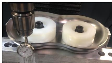
outside machining on half cells for full penetration weld
