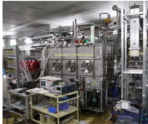
**cERL Injector cryomodule**
