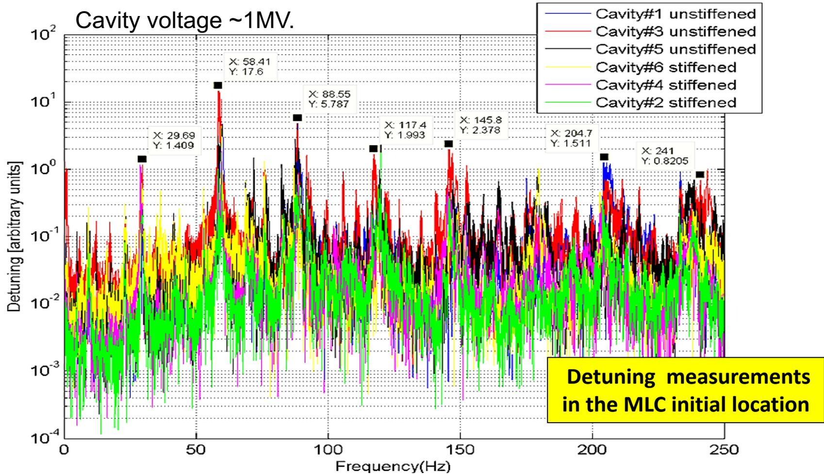
The spectrum of mechanical resonant : 30Hz, 60Hz, 90Hz, etc.
