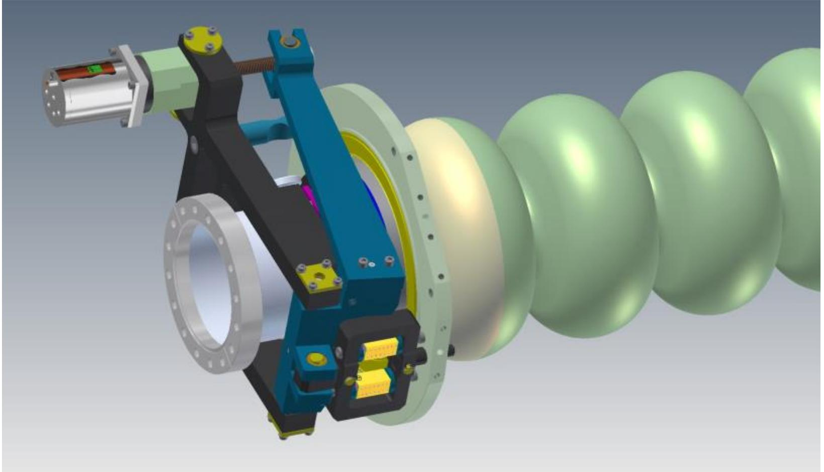
**MLC Cavity Tuner Mounted on an Un-stiffened Cavity Helium Vessel**
