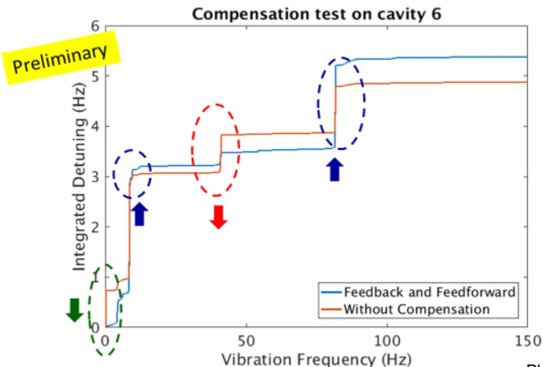
The first attempt of microphonics feedforward compensation on cavity#6.
