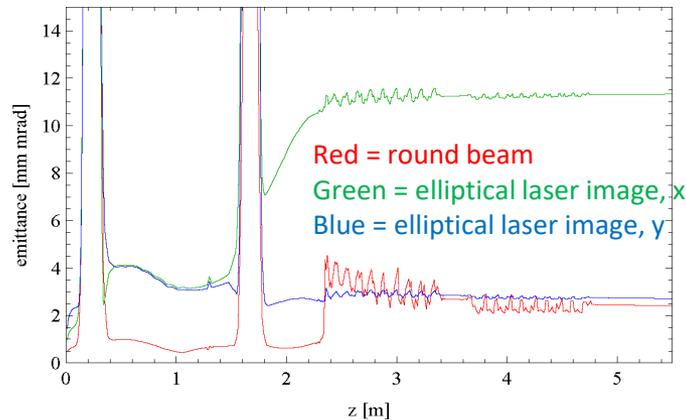
2014 realignment in laser transport led to round spot and subsequent emittance improvement
