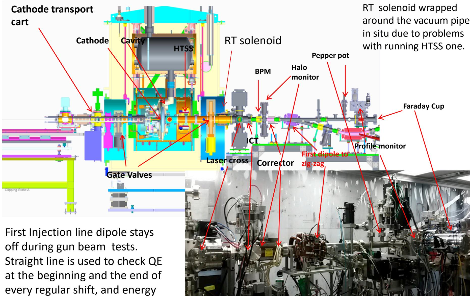
First Injection line dipole stays off during gun beam tests. Straight line is used to check QE at the beginning and the end of every regular shift, and energy measurements.
