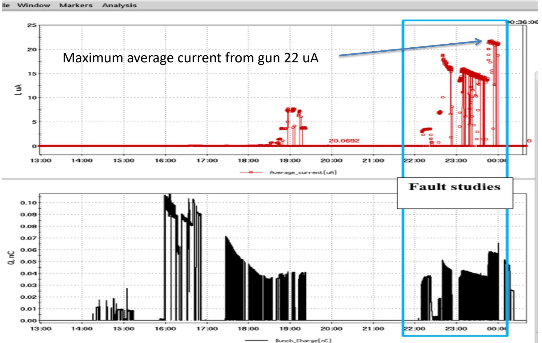
Average current and charge from the gun during fault studies measured by ICT and pulse counter.
