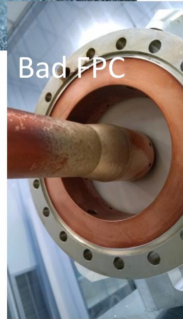
When cavity has been opened and copper marks have been observed at niobium part of chock join. Presumably cavity has been contaminated during severe cathode stalk RF conditioning.
