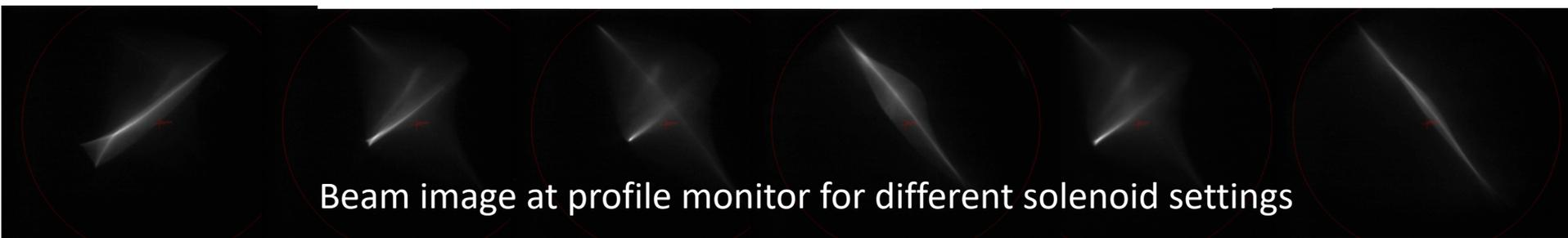
Beam image at profile monitor for different solenoid settings
