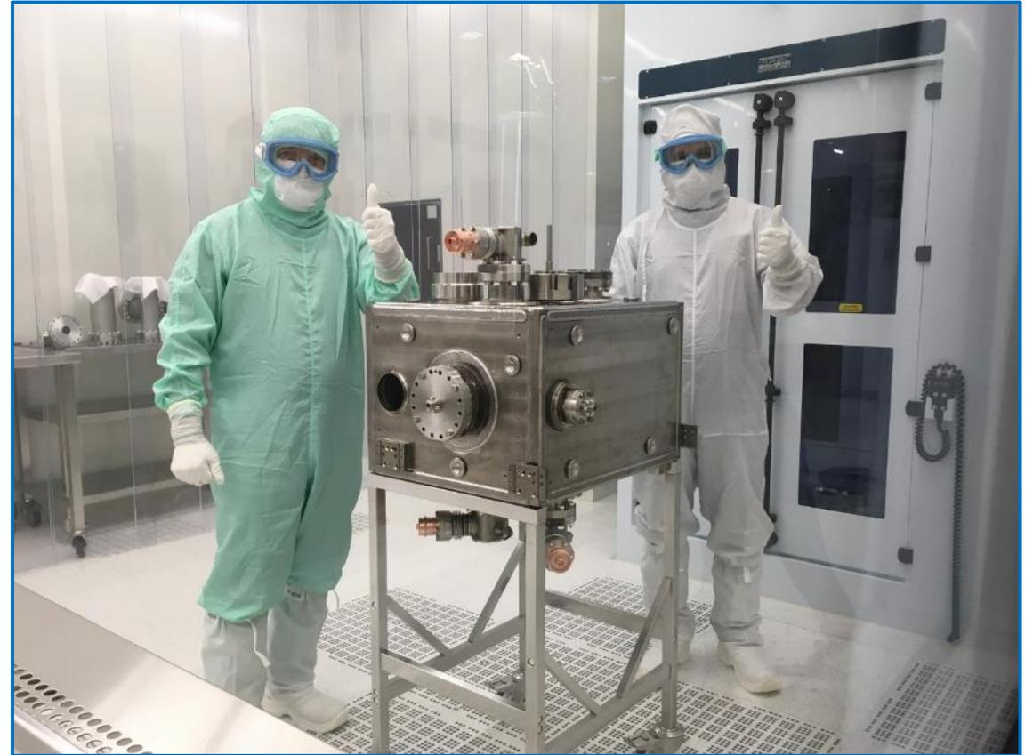
Mounting of the HL-LHC crab HOM couplers with accura 25 3D printed guiding systems in ISO 4 clean room
