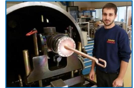
Brazing, EB welding, laser welding, are key processes for the FPC
