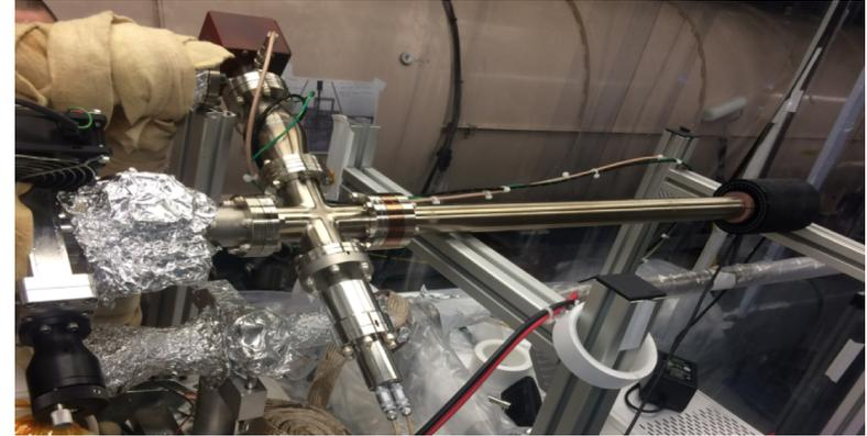
112 MHz gun cathode transferring chamber
