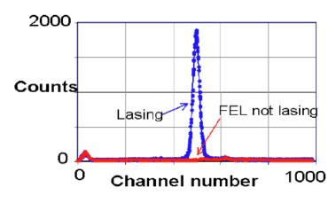
Measured 5.12 keV X-ray Spectrum (Tunable from 3.5 to 18keV)
