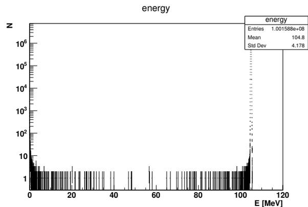
Figure 3: Electron energy spectrum after target passage. At beam energy are no visible changes, while few low energy particles are produced through scattering.
