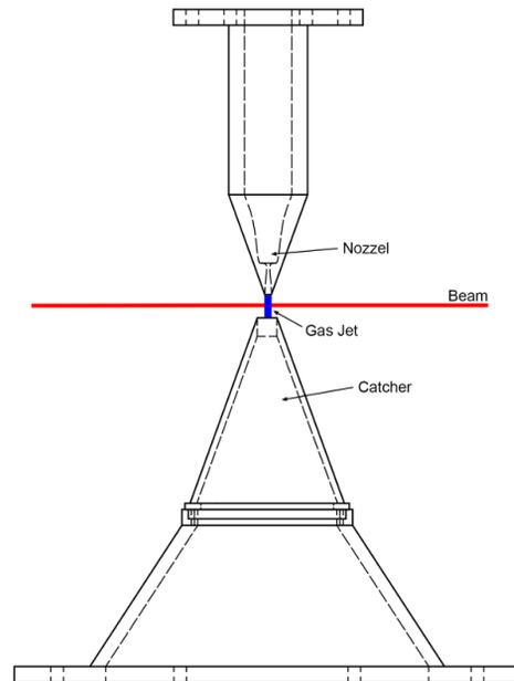
Figure 1: Schematic drawing of the MAGIX gas target [6].
