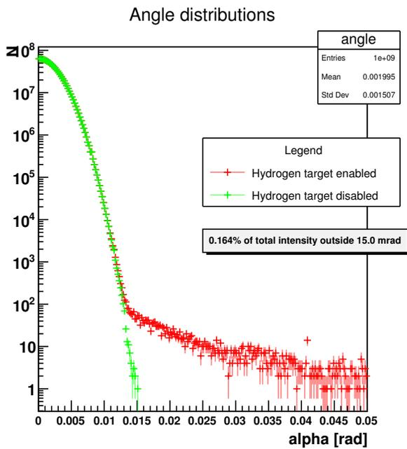
Figure 2: Geant4 simulation of the angle distributions with (red) and without (green) a hydrogen target as designed for MAGIX. TAIL region starts at 15 mrad.
