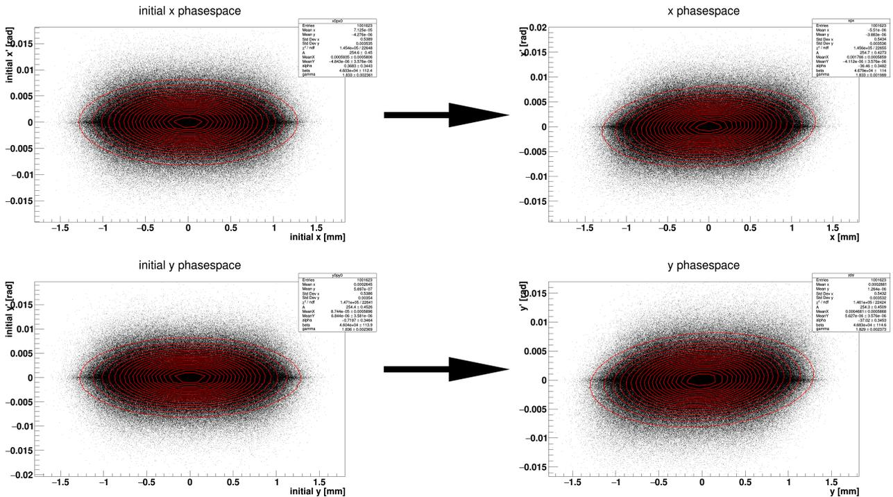
Figure 4: Transverse phase spaces before (left) and after target passage (right). The red RMS ellipses are fitted and show no RMS emittance growth.
