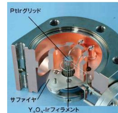
Special RGA ion source for XHV
