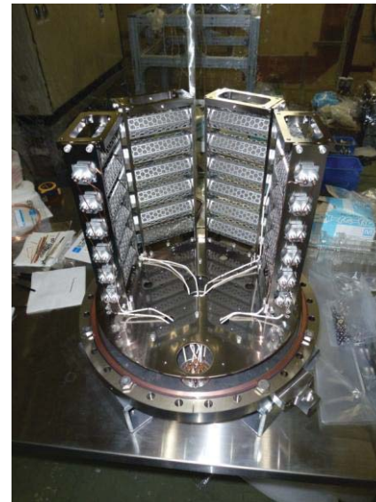
NEG pump set
