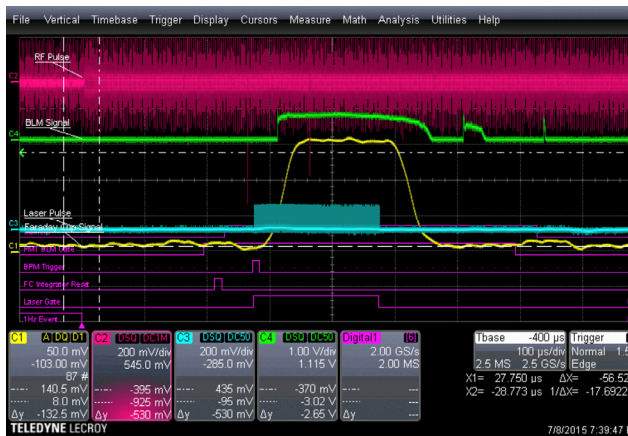
Figure 5: DCCT response to 200 \mu s long macrobunch; DCCT signal on yellow trace, pulse train on blue trace.
