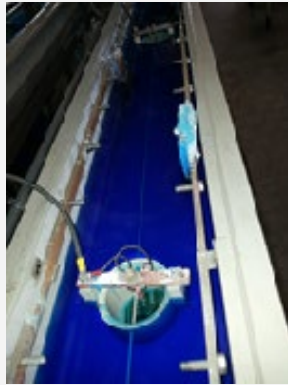
Ti-MgB 2 tape during copper plating
