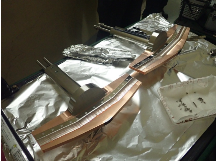
Attach RF-fingers to the spare jaws.
