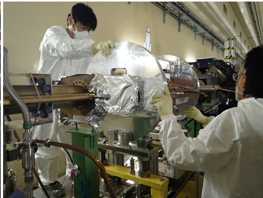
Remove the beam-pipes nearby, and rotate the chamber 90 degrees
