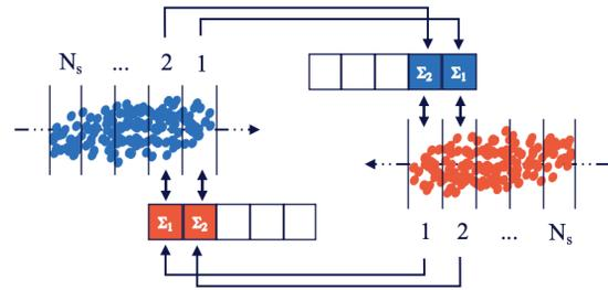
Figure 1: Modelling of beam-beam collision in a numerical tracking code, using the Lorentz-boost approach. Note the difference in the transverse offset between the head and the tail of the bunches.
