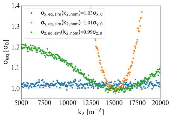
Figure 7: Simulated equilibrium weak bunch sizes as a function of the geometrical crab-sextupole strength  $k_2$  at the FCC-ee Z resonance. The values are always normalised to the nominal equilibrium (=initial in this case) bunch sizes.
