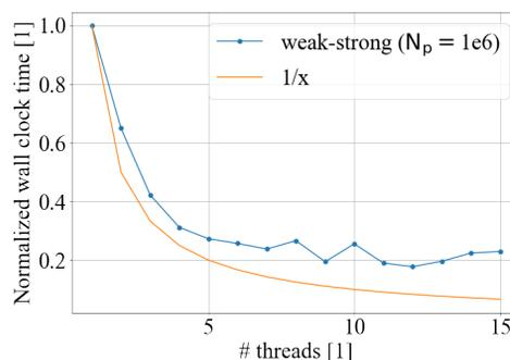
Figure 3: Integrated wall clock time as a function of the number of compute threads for a set of weak-strong simulations (including a linear half-arc) with the FCC-ee Z parameters, each tracked for 100 half turns.
