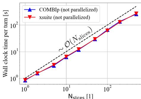
Figure 2: Simulated average wall clock time per turn of the strong-strong beam-beam model as a function of the number of longitudinal slices for `xsuite` (red) and the reference code COMBIp (blue).
