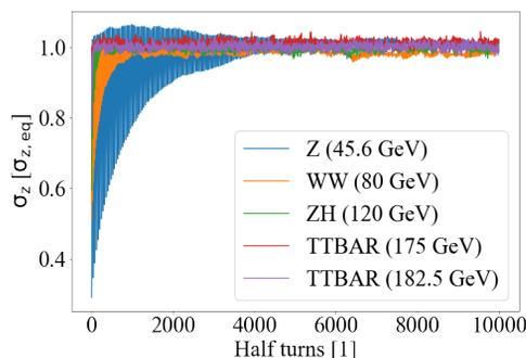
Figure 6: Evolution of weak bunch length for all FCC-ee energies. The values are always normalised to the nominal equilibrium bunch length, taken from [1].
