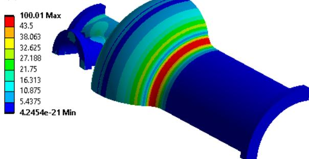
Figure 5. Tuning deformation of 591 MHz 1-cell cavity.
