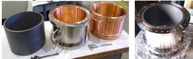
Figure 19. Dielectric beam line absorber with shrink-fit cooling jacket.
