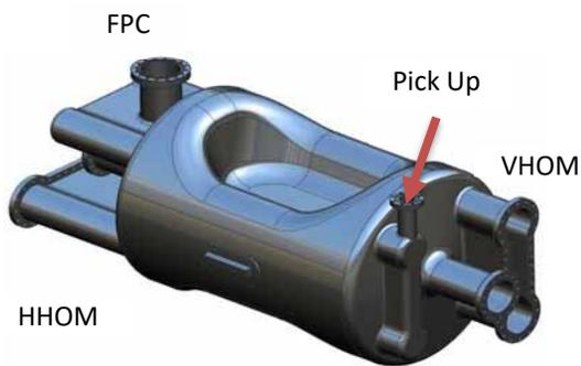
Figure 9: 197 MHz RFD type crab cavity.
