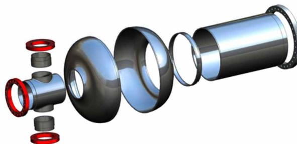
Figure 8: Fabrication model of the 591 MHz 1-cell SRF prototype cavity.
