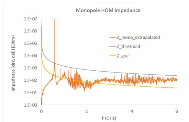
Figure 3: Monopole impedance of asymmetric 591 MHz SRF cavity.
