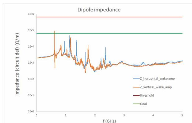
Figure 4: Dipole impedance of asymmetric 591 MHz SRF cavity.
