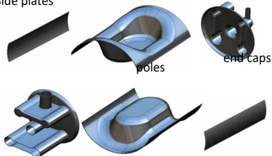
Figure 17. Major high-level subassemblies of the 197 MHz crab cavity prototype. Each assembly will be made from several smaller parts.
