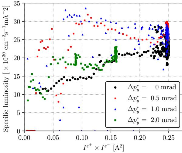
Figure 5: Specific luminosity as a function of beam current products with different four vertical crossing angle at IP.
