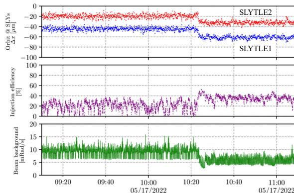
Figure 13: Tuning of orbit at SLYs with a localized orbit in HER, where time histories of orbit at SLYs, injection efficiency and BG are shown.
