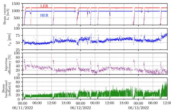
Figure 15: Degradation of machine performance within a few days in HER, where time histories of stored beam current, vertical emittance, beam injection efficiency and BG are shown.
