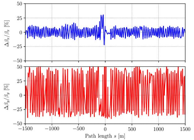
Figure 7: Measured beta-beating in LER. The measurement was performed on May 21st, 2021.
