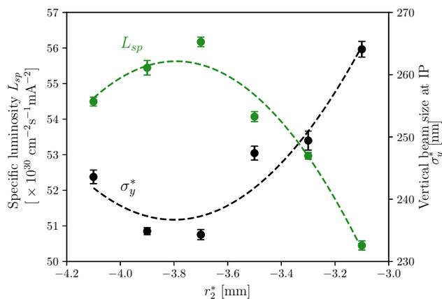
Figure 4: Specific luminosity and vertical beam size as a function of  $r_2^*$ .
