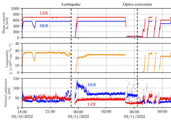
Figure 14: Machine parameters before and after an earthquake. Time histories of stored beam current, luminosity and vertical emittance are shown.
