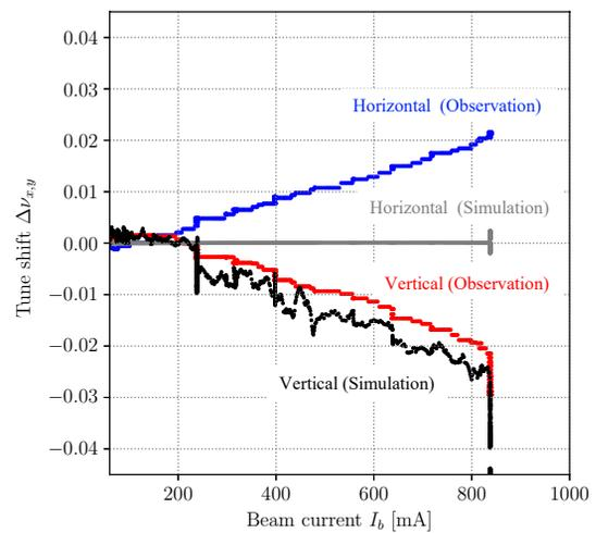
Figure 10: Current dependent tune shift estimated by orbit at SLYs together with that of observation.
