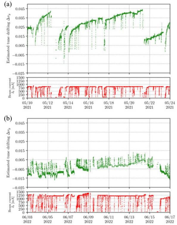
Figure 6: Vertical tune drifting in LER estimated with amount of tune feedback in 2021 (a). Tune drifting is reduced in 2022 by the modification for the ramp cycle of QCS
