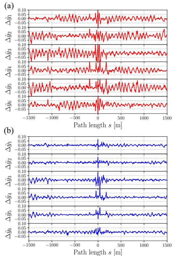
Figure 2: Measured vertical leakage orbits in HER before (a) and after (b) the optics correction. The vertical axis is normalized by root-mean-squared (RMS) amplitude of the horizontal orbits. IP is located on  $s = 0$ .
