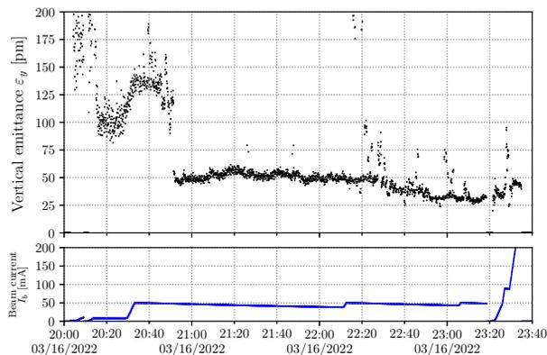
Figure 3: Time evolution of the vertical emittance together with beam current in HER during a series of optics correction.
