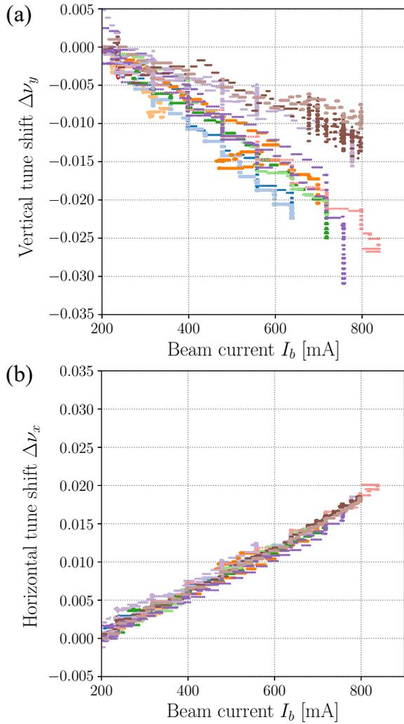
Figure 8: Horizontal (a) and vertical (a) tune shifts estimated by the amount of tune feedback as a function of stored beam current in HER. Each marker represents a measurement day.
