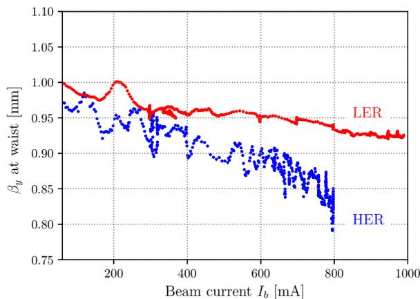
Figure 12: Estimated vertical betatron function at IP as a function of stored beam current.
