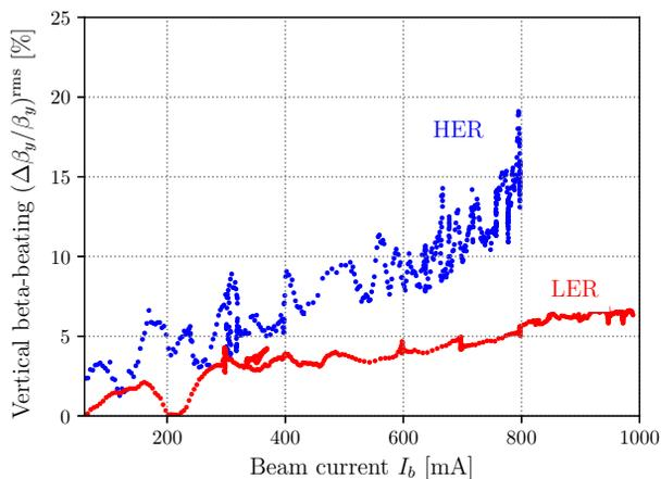
Figure 11: Estimated vertical beta-beating as a function of stored beam current, where the residual beta-beating is calculated with root-mean-squared of beta-beating at all BPMs.
