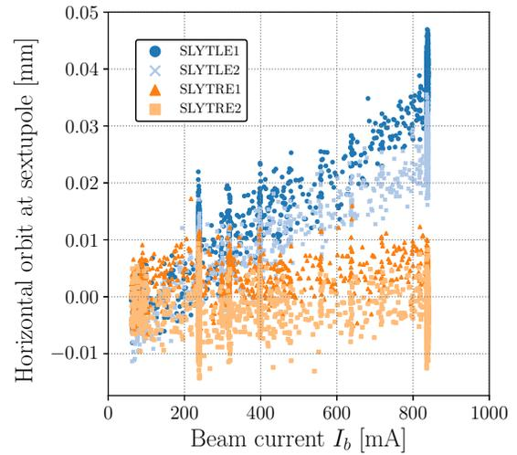
Figure 9: Horizontal beam orbits at SLYs (SLYTLE1, SLYTLE2, SLYTRE1 and SLYTRE2) and stored beam current in HER.
