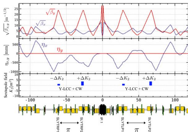
Figure 1: Betatron and dispersion functions at the Y-LCC section in LER. Two sextupoles pairs installed in both left and right sides of the interaction region. The sextupole pairs are utilized for Y-LCC and CW. Betatron phase advance between the two sextupoles is  $\pi$ .
