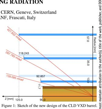
Figure 1: Sketch of the new design of the CLD VXD barrel. The blue shapes represent the dimensions of the layers in the new version, the light blue shapes refer to the CDR version. The gold shape is the beam pipe central chamber.
