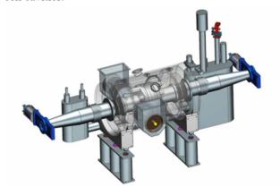
Figure 1: Symmetric single cell 591 MHz SRF cryomodule with two large warm BLA's and tapers in the CDR.
