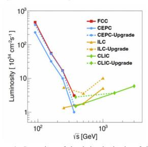
Figure 1: Comparison of the design luminosity of the CEPC and those of other electron-positron Higgs factories.
