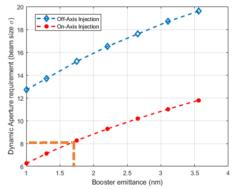
Figure 1: The dynamic aperture requirement of collider ring in horizontal direction due to injection process vs. booster emittance at 120 GeV. The horizontal emittance in collider ring at 120 GeV is 0.64 nm. The horizontal beta function at the injection point is 1800 m.
