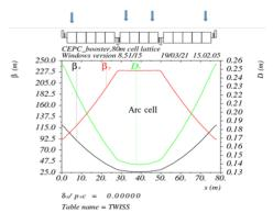
Figure 2: The Twiss functions of the TME cell in the arc region.
