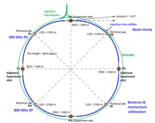
Figure 1: Schematic layout of the FCC-ee collider with a circumference of 91.1 km and four-fold superperiodicity. The full-energy booster and part of its injection transfer line are also indicated.
