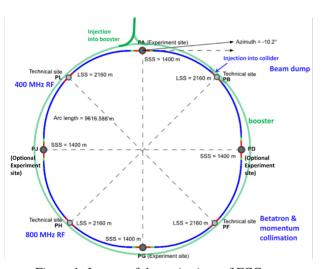
Figure 1: Layout of the main rings of FCC-ee.
