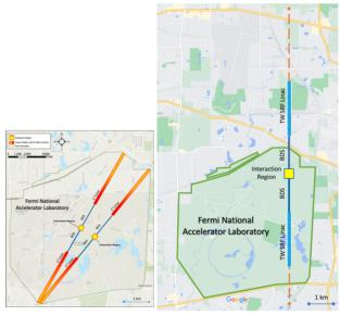
Figure 1: Possible placements of future linear  $e^+e^-$ Higgs/EW factory colliders  $C^3$  and HELEN on the Fermilab site map - both about the same length: (left) 250 GeV c.m.e. options with a 7-km footprint, and (right) higher c.m. energy options (12 km dashed line) (from the AF report [2]).
