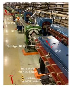
Figure 2: Photograph of an arc-section of the SuperKEKB main ring.
