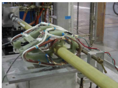
Figure 3: Ante-chamber type dithering coil is being measured by a rotating system.
