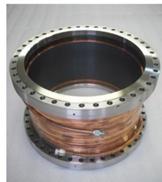
Figure 2: A KEKB type LBP damper with 4-mm thickness of ferrite, \phi 300 mm, length of 150 mm.
