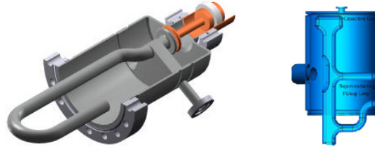
Figure 24: Original and later, modified hook type coaxial HOM couplers.
