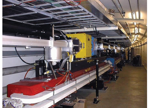
Figure 1: PEP-II tunnel with LER above the HER with injection in the vertical plane.
