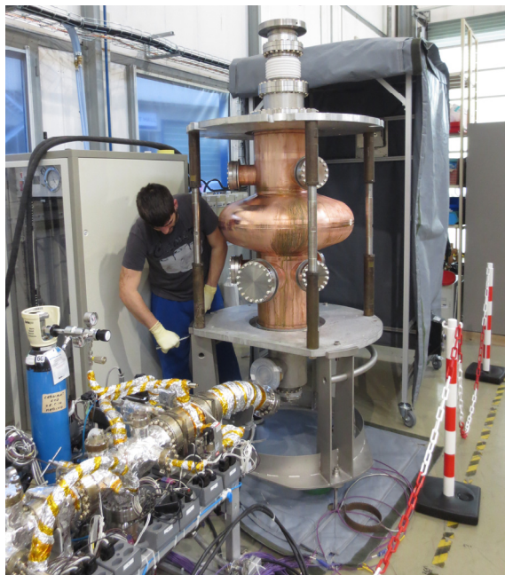
Figure 29: LHC spare cavity assembly for Nb coating.
