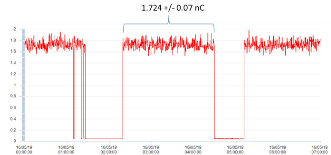
Figure 12: Beam charge stability of RF gun.
