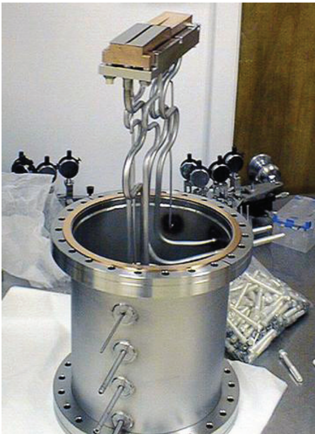
Figure 14: HER synchrotron light mirror with main power slot down the center to reduce mirror distortions.
