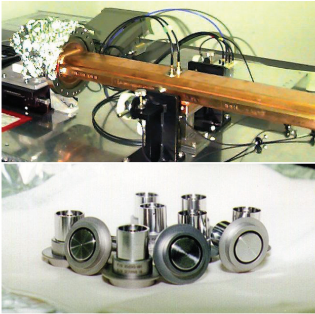
AF_002 Pick-up Buttons for the Beam-Position Monitors 8-19-97
