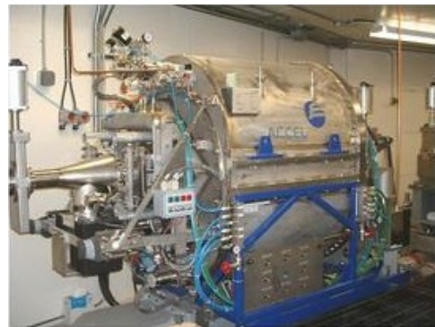
Figure 1: CESR-B type 500 MHz cavity cryomodule produced by Industry.
