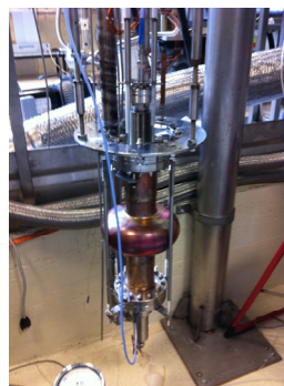
Figure 31: CERN HIPIMS cavity coating system and QPR sample test cavity concept.
