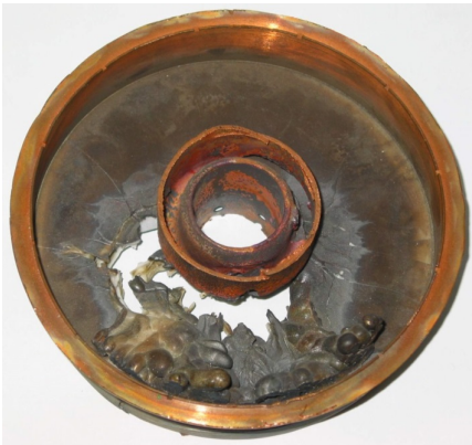
Figure 22: Example of coaxial power window failure due to arcing.
