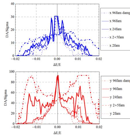
Figure 2: The dynamic apertures of CEPC PDR [2] in  $x$ - $z$  (top) and  $y$ - $z$  planes (bottom). The lines show the difference between the number of sextupole families. The largest ones include synchrotron radiation damping, and are approaching the goal momentum aperture  $\pm 2\%$ .
