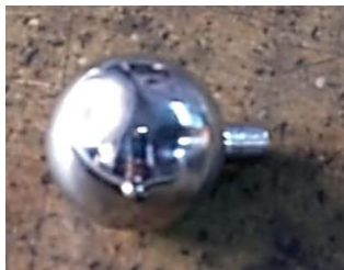
Detachable spherical 1-inch (2.54cm) diameter Langmuir probe head
