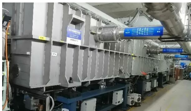
Super-conducting linear accelerator (CW - linac)
