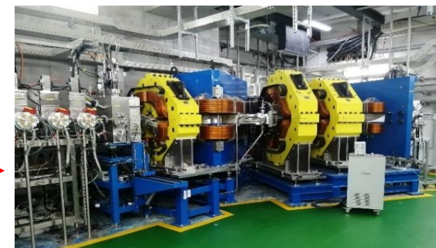
Gas-filled recoil separator (SHANS2)
