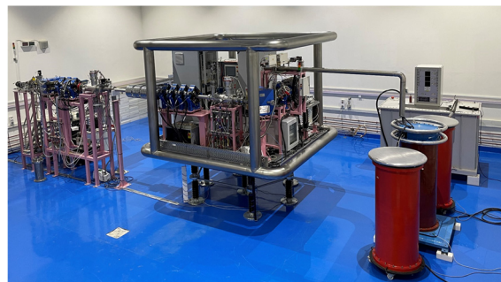
Figure 1: Photograph of Accelerator based 14 MeV Neutron Generator.
