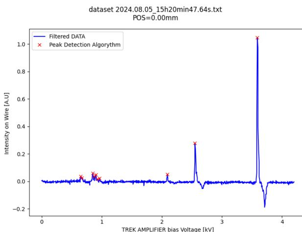
Figure 3: Mass spectrum of ALISES v2 at 35 keV.
