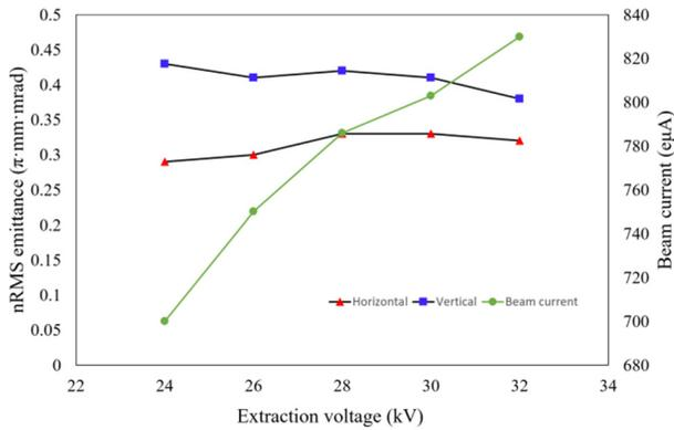
Figure 5: C<sup>4+</sup> beam emittance versus extraction high voltage.
