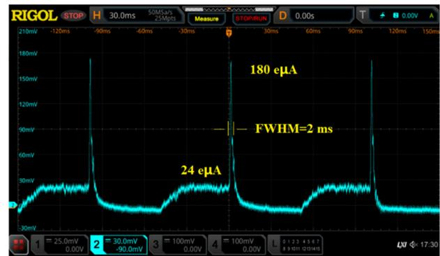
Figure 3: Afterglow mode test on C<sup>5+</sup> ion beam.
