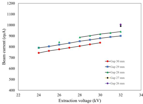
Figure 4: C<sup>4+</sup> beam current versus extraction high voltage with different extraction gap.
