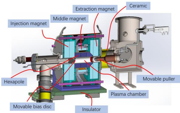
Figure 2: Structure of the LAPECR3 ion source.
