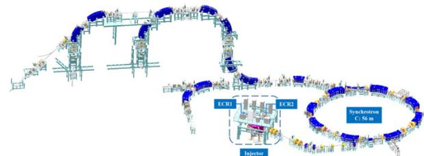
Figure 1: Schematic layout of HIMM facility.
