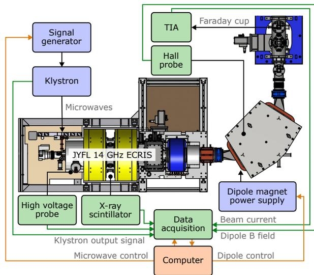
Figure 1: A schematic of the experimental setup.
