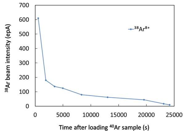
Figure 3: Decay curve of <sup>38</sup>Ar on the proxy FC following ECR3 operation with enriched 99.96% <sup>38</sup>Ar gas at 235 enA on the same FC.
