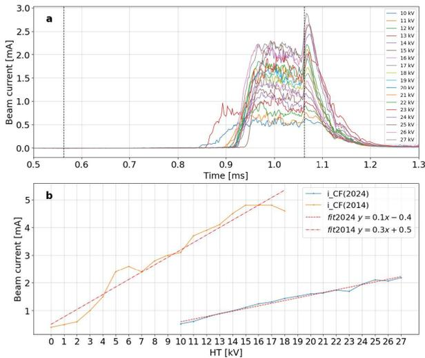
Figure 2: (a) Temporal evolution of the total beam intensity measured in FC-Source for various source high voltage, with a RF power of 80 kW. (b) Evolution of the average ion pulse current as a function of the source high voltage for the 2014 data (orange) and the 2024 data (blue).
